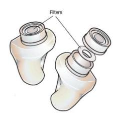
The vented/tuned earplug, which does not reduce sound levels up to about 2000 Hz, reduces higher frequencies significantly. Typically, vented/tuned earplugs attenuate higher frequencies by about 20 dB when the adjustable vent is wide open. Closing the vent increases higher-frequency attenuation to as much as 28 dB (performance similar to compressible earplugs). Most ear-mould laboratories can make custom-moulded vented/tuned earplugs.
